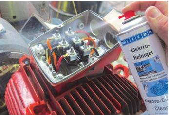
Electro Contact Cleaner reduces voltage losses and increases the electric conductivity. Contamination that can cause tracking current is removed.
