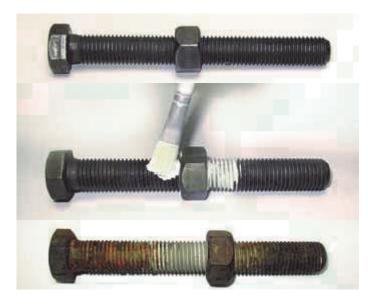
Due to the special formulation and the very fine grinding of the solids contained in Weicon Anti-Seize, irregularities in the surface to be protected (even to a thickness of only 12  $\mu$ m) are completely filled. Only a perfectly sealed surface guarantees reliable protection against corrosion.
