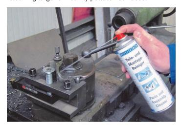
Due to the high flash point (>60°C for the active substance) this cleaner corresponds to the former German Vbf-classification AIII and complies with the cooperative recommendations for safety at work. This is an advantage when compared to AI or AII cleaners.
