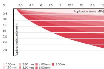
A Load Deflection (LD) curve is a Stress (MPa) vs. Strain (mm) curve. It is the load required to compress a material at a defined thickness for a determined deflection. Its commonly used when making material selections to meet engineering requirements such as flange load or controlled compression applications.
