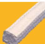
**Marigold 344BIL** is braided from 100% pure PTFE filament and has been thoroughly impregnated with a PTFE suspensoidal blocking agent and a proprietary break in lubricant. A soft but dense and stable packing, the unique blend of lubrication in 344BIL eases friction during both start-up and operation making it well suited to environments requiring extremely low shaft friction along with excellent resistance to aggressive chemicals.
