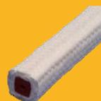
**Marigold 344FDA** is braided from 100% pure, continuous PTFE fibres that satisfy all (US) FDA requirements for food contact. It is typically used in the food processing industry or anywhere a FDA approved packing is required for pumps or valves.
