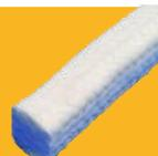
**Marigold 344-SC** is an interlock braided packing manufactured from 100% pure PTFE filament, impregnated with a PTFE blocking agent and braided around a silicone core. The silicone core increases compression recovery and helps account for shaft deflection to ensure a tight, long lasting seal. Typically used in chemical applications with worn or bent shafts, Marigold 344-SC has an extremely low coefficient of friction and excellent heat dispersion.
