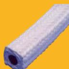
**Marigold 344BIL-SC** consists of pure PTFE filament, a PTFE blocking agent and our proprietary break in lubricant all braided around a silicone core. The break in lube reduces friction during start-up and operation whilst the durable silicone core improves compression recovery and reduces the impact of worn shafts and shaft deflection. 344BIL-SC is used on chemical pumps requiring low friction and high chemical resistance.
