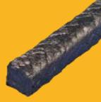
**Marigold 5000-OCC** is similar to 5000C as both are constructed from high purity graphite yarns reinforced with high strength carbon filament. The difference between these two styles is in the braid type used; Marigold 5000-OCC is interlock braided whilst 5000C is plait. The stronger interlock braiding allows 5000-OCC to be used in extremely high pressure environments whilst the unique blend of materials used ensures it offers many of the outstanding performance attributes of Mari-
