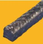
**Marigold 5000C** is a plait braided packing manufactured from high purity graphite yarns and reinforced with high strength carbon filament. Highly durable and easy to install, this low leakage packing is self-lubricating and offers superior extrusion resistance. The unique blend of carbon and graphite used in its construction ensures extremely low shaft wear and excellent heat dissipation. Marigold 5000C is used in air up to 455°C, steam to 649°C and in non-oxidising atmospheres up to 3315°C.
