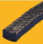
**Marigold 5000T** is manufactured from high purity graphite yarns combined with a densified PTFE dispersion. This interlock braided packing is used in applications with high pressures and aggressive chemicals and has been widely utilised on a variety of pump and valve types. Marigold 5000T is a self lubricating packing with excellent extrusion resistance. The unique blend of PTFE and graphite ensures 5000T offers extremely low shaft wear whilst maintaining its excellent heat dissipation.
