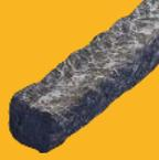
**Marigold 8000LC** is an interlock braided pump and valve packing produced from industrial grade graphite filaments and coated with a proprietary graphite blend. This addition coating ensures Marigold 8000LC has a low coefficient of friction and that fraying is minimised. Used in sealing highly aggressive media, Marigold 8000LC exhibits extremely high rates of thermal conductivity and in air up to 455°C, steam to 649°C and in non-oxidising atmospheres up to 3315°C..
