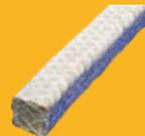
**Marigold 320** is an interlock braided packing produced from Kynol and impregnated with PTFE and our proprietary, inert, break-in lubricant. The phenolic fibres used in Marigold 320 produce a packing which is non-staining, non-hardening and highly durable that offers low shaft wear and low leakage rates over a long service life. Marigold 320 is a general purpose packing used in pump and valve applications requiring a economical and highly durable packing which still offers good conformability.
