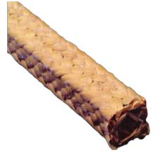
Description: Aramid filament is impregnated with PTFE and an inert lubricant then braided into a dense, resilient packing.
